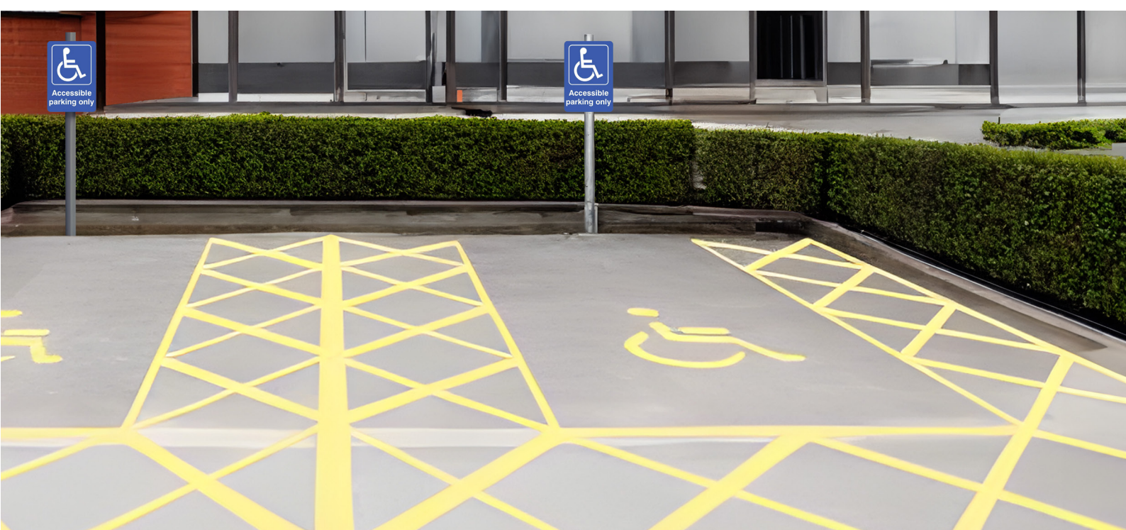
Illustration of a disabled parking bay with a clear area on three sides
